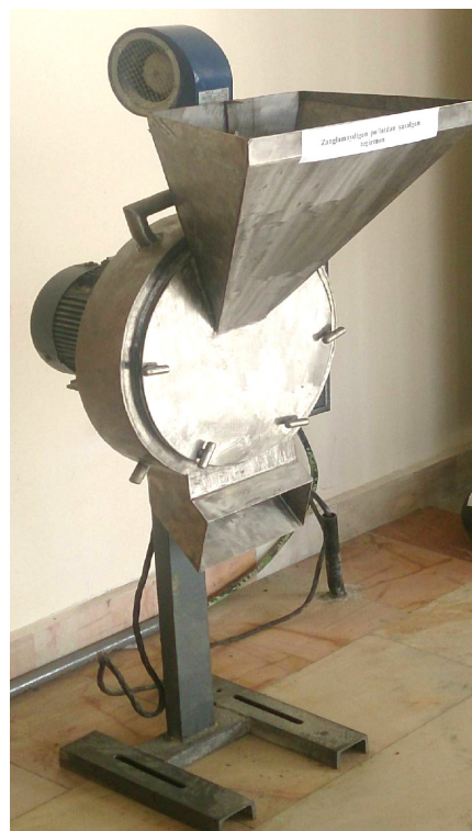
Fig. 1. Appearance of developed a hammer mill with a system of water and air cooling of stainless steel
