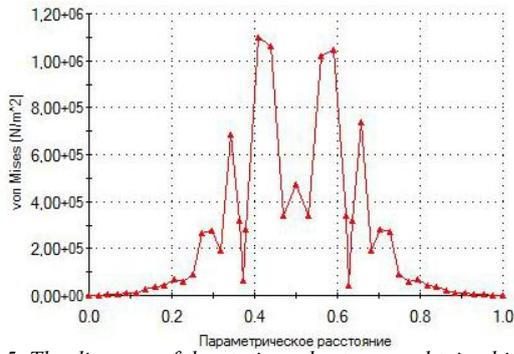
Fig. 5. The diagram of the static node stresses obtained in the simulation loading of workpiece with line microdisplacements of tongs (a) and turning (b)
