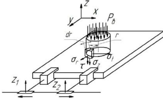
Fig. 1. The layout of waterjet cutting machine with a movable workpiece and movable jet head in a vertical plane (fixed in the plane XOY)
