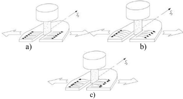
Fig. 2. Creation of stress state of the workpiece in the cutting zone with longitudinal loading by force R (a) and loading momentum M relative to OZ (b), the combined action of the force and momentum (c)
