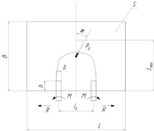
Fig. 3. Captures with microdisplacements drives (a) and the calculation scheme of sheet blank with preload area (b)
