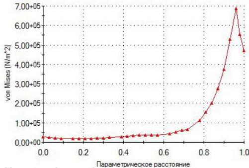
Fig. 6. Changing the tensile stress along the OY on symmetry axis of the drive (shown relative distance in the horizontal, coordinate origin at the right edge)
