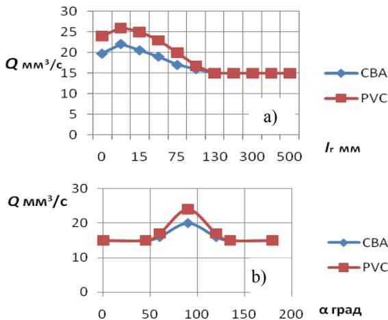
Fig. 7. Change of productivity, expressed as the volumetric material removal at waterjet cutting depending on the distance from the edge of tongs (a) and the angle between the tangent to the contour of the cut and the axis of symmetry of the working body (b)
