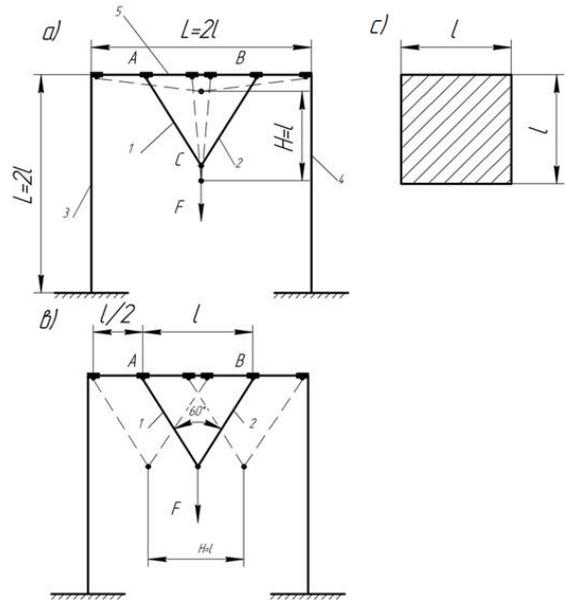
Fig. 4. The diagram of floor-mounted industrial robot with flat PSM of biglide type and the manipulated object moving in vertical (a), horizontal (b) directions, forming a square working area (c).
