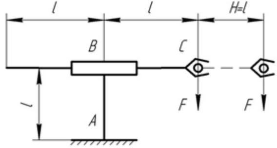
Fig. 3. The diagram of a floor-mounted industrial robot
