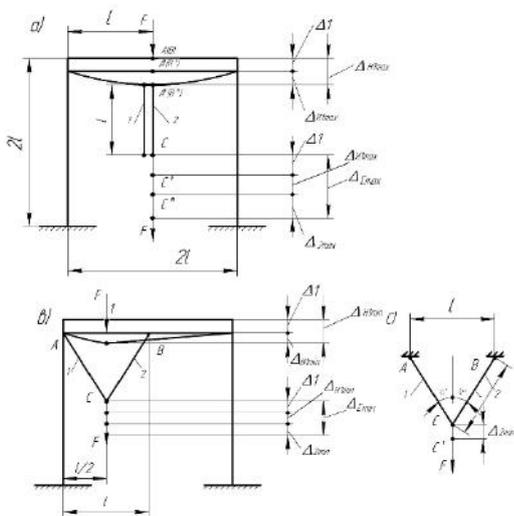
**Fig. 5.** Calculation models for determination of instability factor for a gantry robot with a biglide PSM (fig. 4) in positions of the maximum (a) and the minimum (b, c) manipulated object elastic displacement in the point C of the force F application area.
