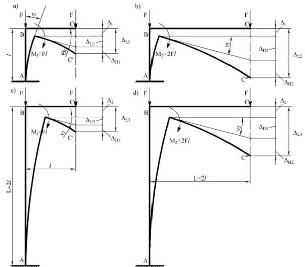
**Fig. 2.** Curved rods (frames) being compared with different part length ratios AB:BC: a - 1:1; b - 1:2; c - 2:1; d - 2:2.
