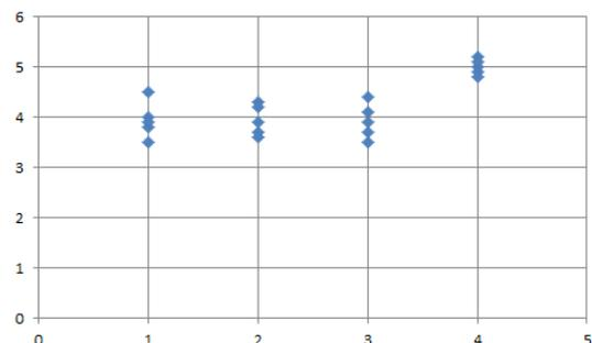
Figure 5 - Changing the growth rate of microcracks from polycyclic controlled load depending on load forms: 1 - quasi-harmonic; 2 - semi-periodic; 3 - stair-step; 4 - sawtooth
