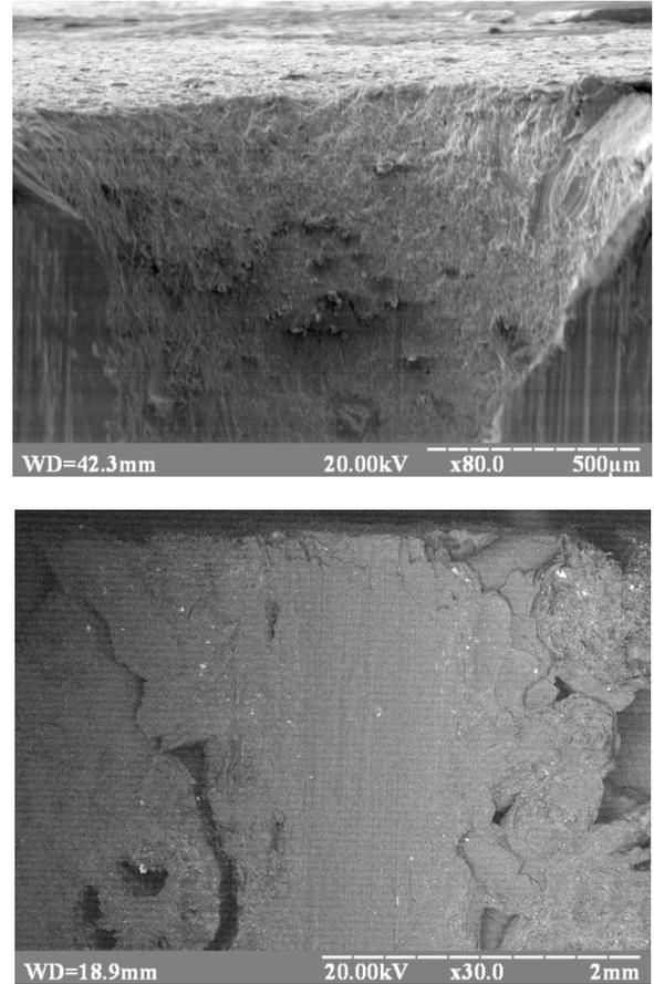
Figure 1 - Formation of cutting hole (a) and cracking (b) in samples of composite workpiece
