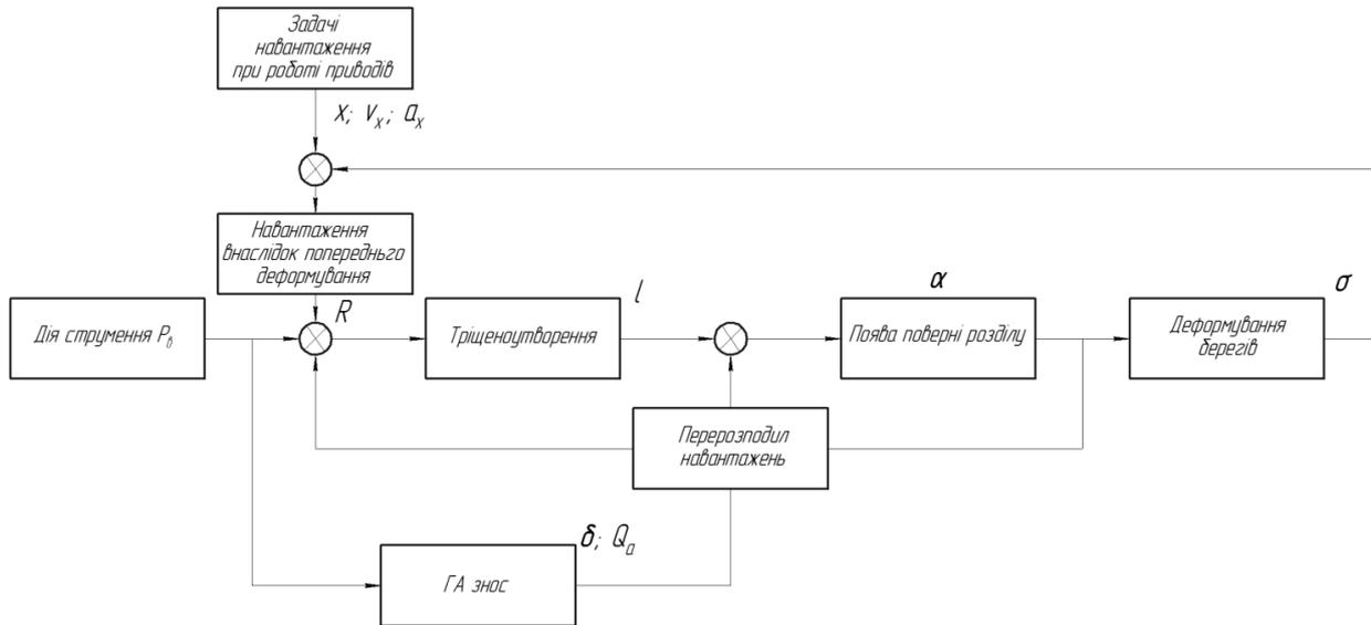
Figure 3 - Block diagram of the process of waterjet cutting of composite with a pre-load of the jet impact zone
