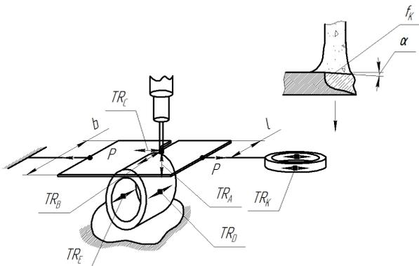
**Figure 6** - The scheme of measurements and photos from the microscope along the length of the cracks
