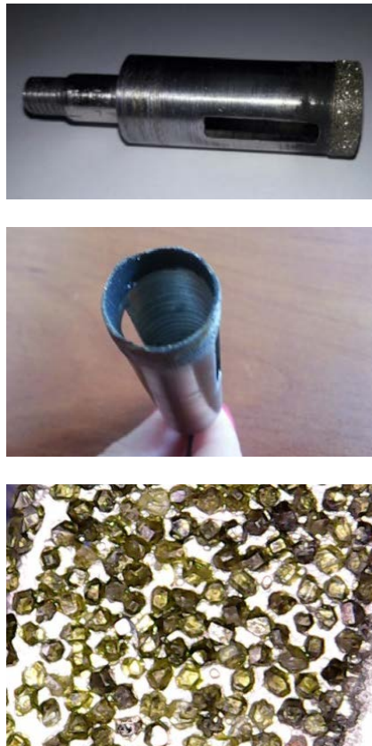
Fig. 15. Special equipment for the drilling (a), drill that used and it geometric parameters (b)
