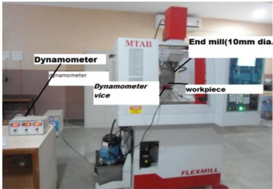
Fig. 4. Experimental milling setup [41]
