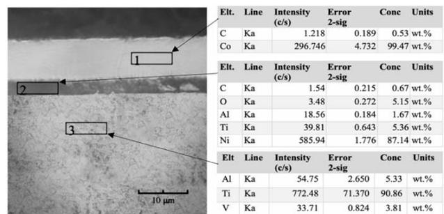
Fig. 2. Chemical composition of zones of cobalt coated Ti-6Al-4V specimen with a bonding layer of nickel
