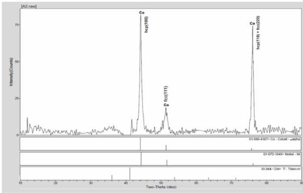
Fig. 3. X-ray diffractogram of the brush plated cobalt coating
