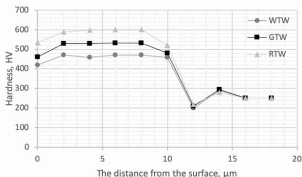
Fig. 6. Microhardness profiles of the Ti-6Al-4V after brush plating of Co with an operating voltage of 12 volts.
