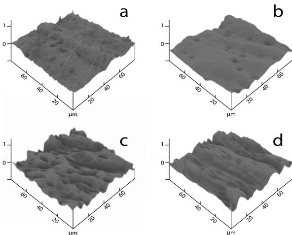
Fig. 4. Surface morphology of the samples of Ti-6Al-4V substrate,  $Ra = 0.036 \mu\text{m}$  (a) and after cobalt brush plating with a different type of electrode cover material: White Tuff Wrap,  $Ra = 0.028 \mu\text{m}$  (b); Gray Tuff Wrap,  $Ra = 0.032 \mu\text{m}$  (c) and Red Tuff Wrap,  $Ra = 0.039 \mu\text{m}$  (d)
