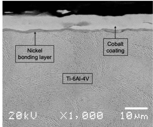
Fig. 1. SEM image of electroplated Ti-6Al-4V sample with a bonding layer of nickel and cobalt coating
