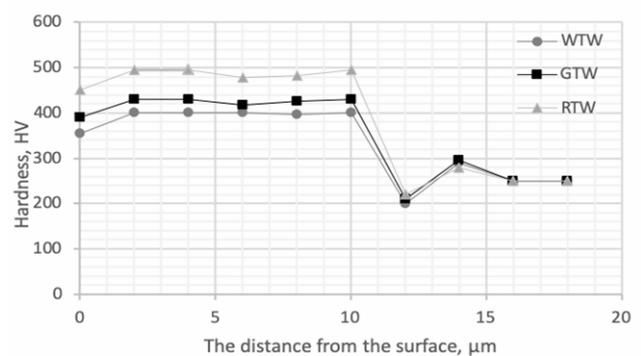
Fig. 5. Microhardness profiles of Ti-6Al-4V after brush plating of Co with an operating voltage of 8 volts.
