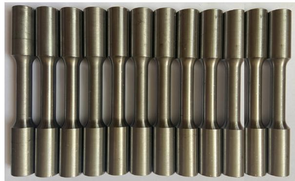
Fig. 2. AISI 4140 tensile test specimens
