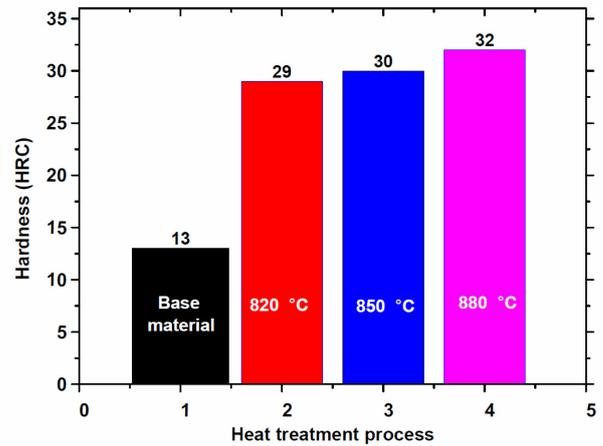
Fig. 6. Rockwell-C hardness graph
