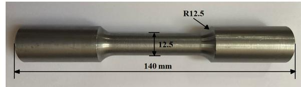
Fig. 1. AISI 4140 tensile test specimen dimensions
