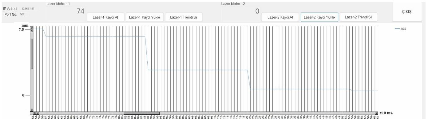
Fig. 10. Triple PZT crystal test specimen's Experimental linear displacement-time result at 220 V Voltage
