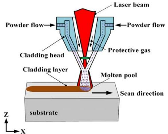
Fig. 1. Schematic representation of laser cladding [8]
