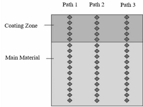
**Fig. 4.** Schematic diagram of the microhardness measurement path
