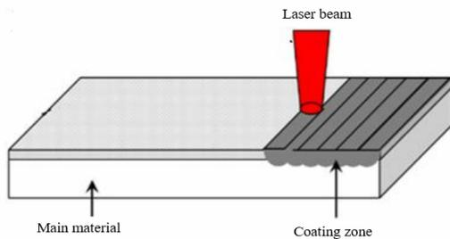
**Fig. 2.** Laser cladding coating method
