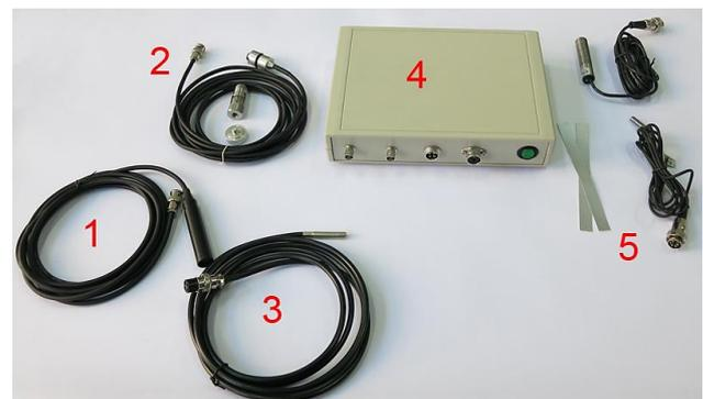
Fig. 4. VibroLog device with sensors
