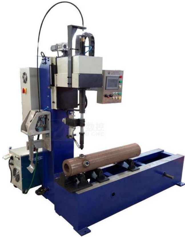
Fig. 2. Automatic welding machine for fittings from the Chinese manufacturer HAOYU [4]
